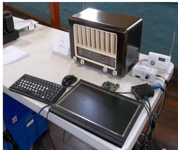
ABOVE: Ian Smyth presented several projects, although his primary project was the restoration of the Phillips radio. Ian rebuilt the dial panel with a piece of glass of a similar vintage, and using screen printing and Photoshop, was able to reproduce the panel layer by layer to a spectacular finish.
