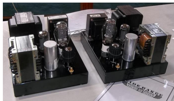
LEFT: Alan Martin with his 5 watt class B amplifier that has no feedback and distortion of 0.1. Originally had problems with a capacitor input which was resolved when changed to an inductive input.
